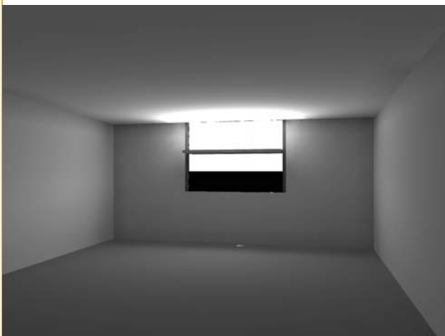
Overcast Sky Daylight Distribution From Light Shelf, h_c = 1/3 H
